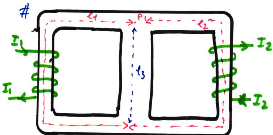
The sectional area of core is  $S_c$ . Determine the magnetic flux in the center leg?
