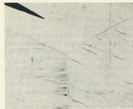
Fig 9. Hot stage microscopy: Growth of Widmanstätten \alpha rods during isothermal ageing the metastable B' phase in a Cu-40% Zn alloy using a hot stage microscope (Ciné film sequence).
