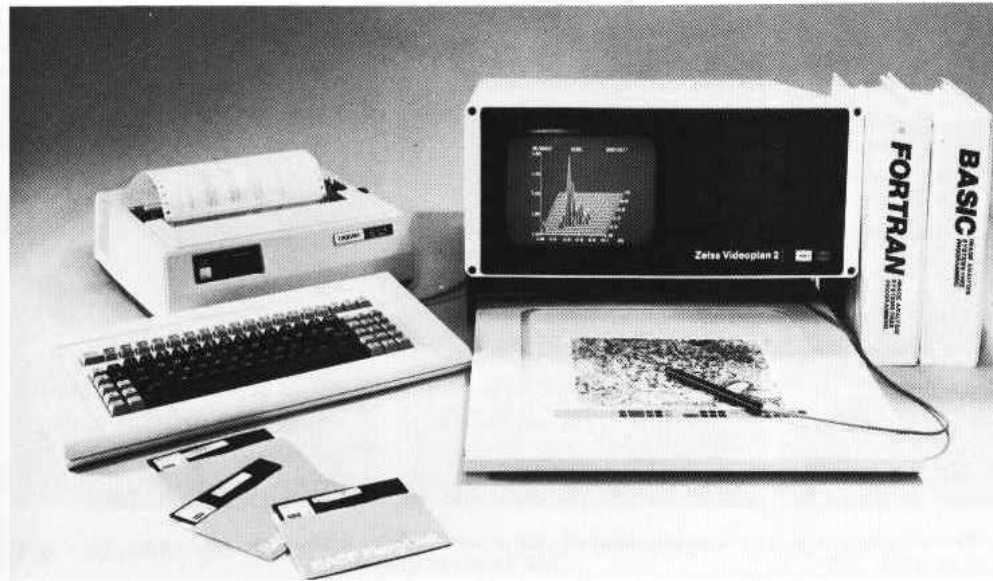
Fig. 49 Semiautomatic image analyzer. With this system, the operator controls detection of features by tracing with a light pen. (C. Zeiss, Inc.)
