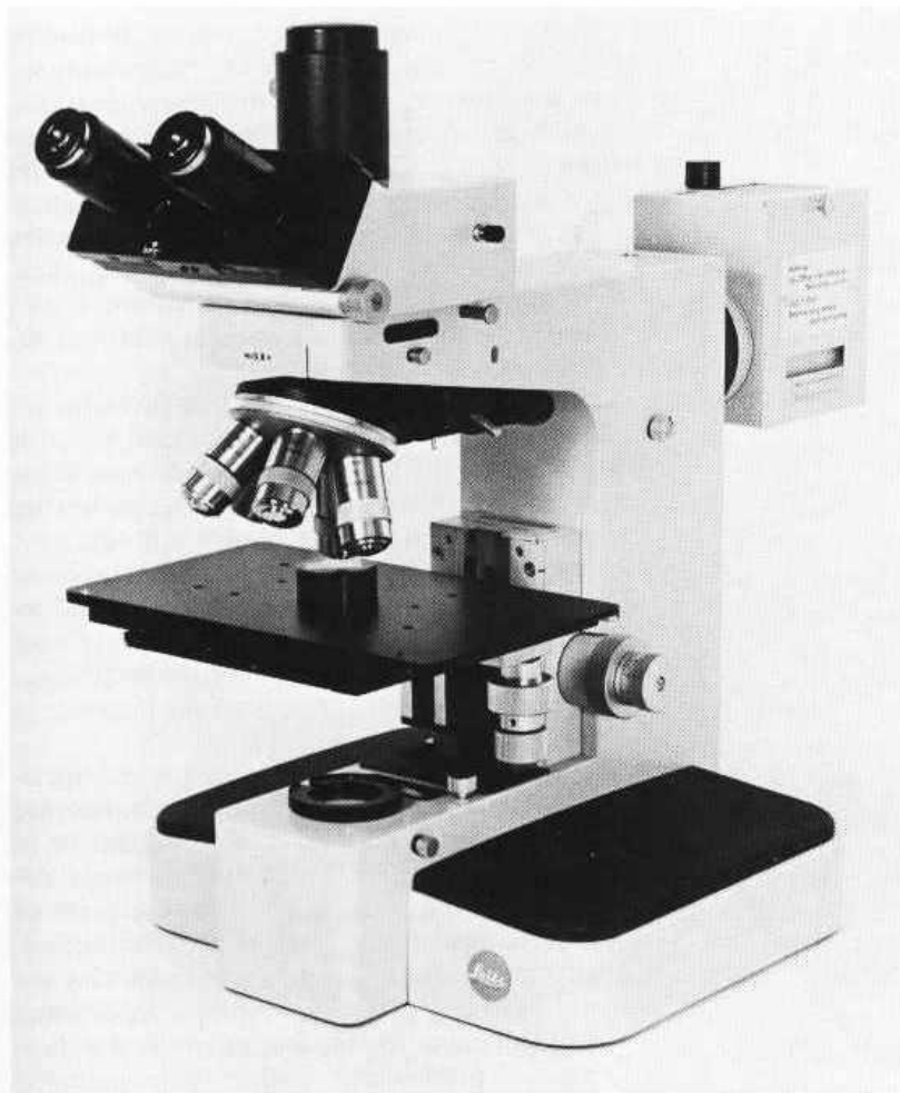
Fig. 3 Research-quality optical microscopes. (a) Upright. (b) Inverted. (E. Leitz, Inc.; Unitron Instruments, Inc.)
