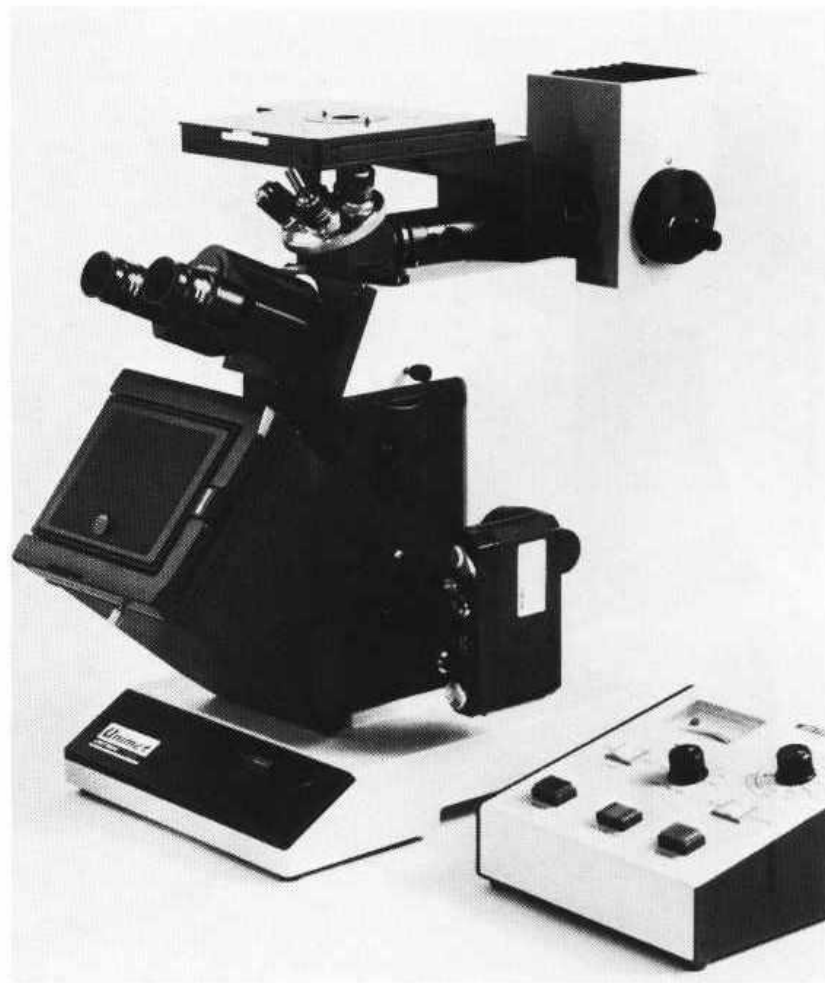
Fig. 3 Research-quality optical microscopes. (a) Upright. (b) Inverted. (E. Leitz, Inc.; Unitron Instruments, Inc.)
