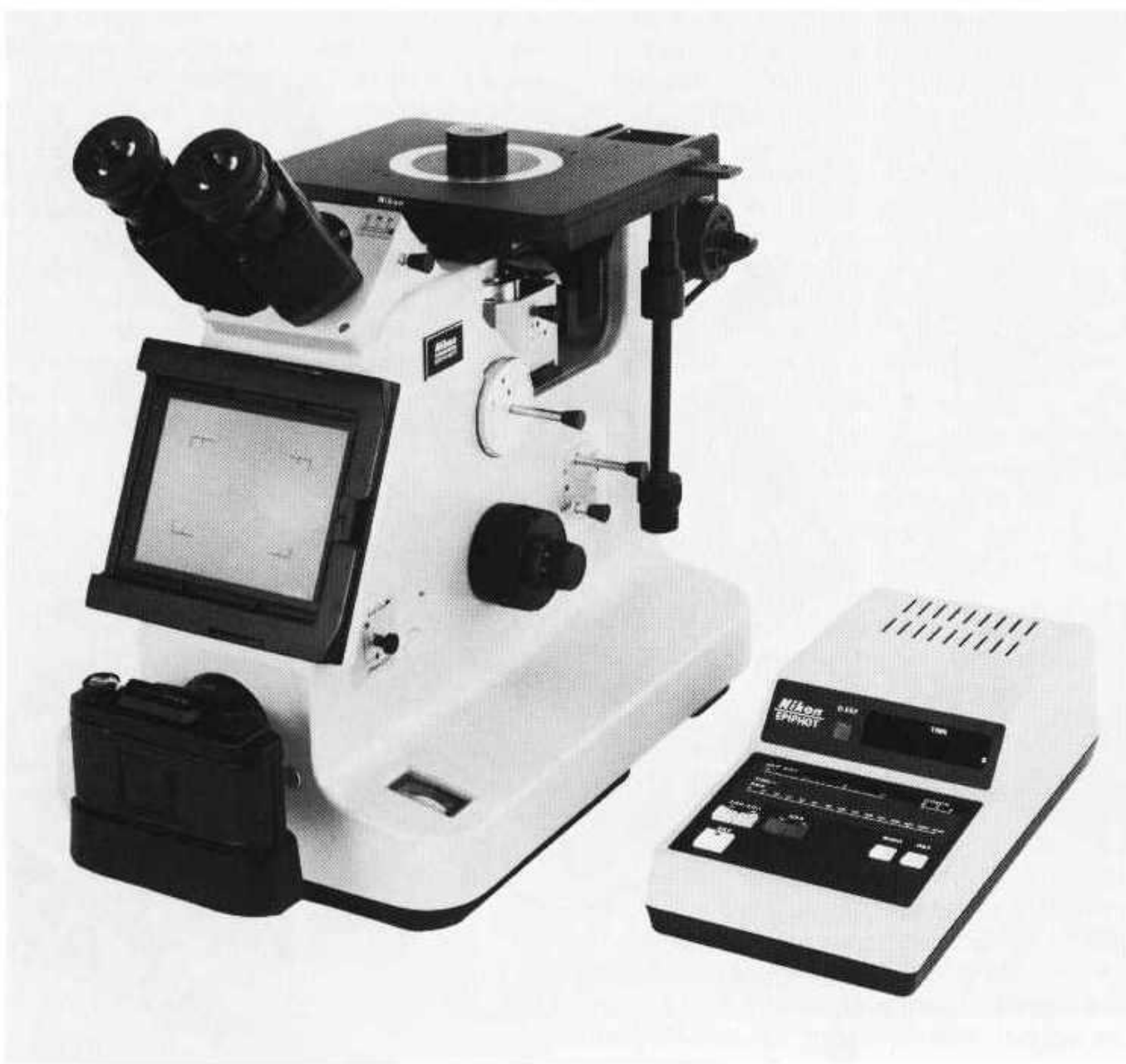
Fig. 4 Moderately priced inverted metallograph. The small box to the right is an automatic exposure control. (Nikon, Inc.)
