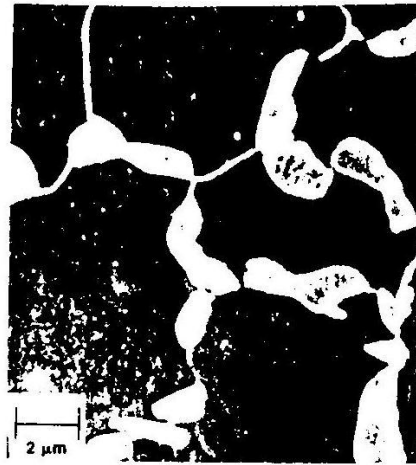
FIGURE 3-37 Ferrite-martensite microstructure of a dual-phase steel (0.06% C, 1.5% Mn); water-quenched from 760°C. The white phase is martensite and the dark phase ferrite.
