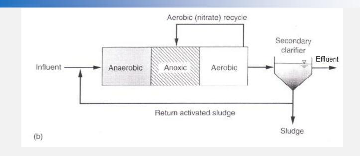
The proprietary A<sup>2</sup>/O process is a modification of the A/O process and provides an anoxic zone for denitrification. The detention period in the anoxic zone is approximately 1 h. The anoxic zone is deficient in dissolved oxygen, but chemically bound oxygen in the form of nitrate or nitrite is introduced by recycling nitrified mixed liquor from the aerobic section. Use of the anoxic zone minimizes the amount of nitrate fed to the anaerobic zone in the return activated sludge
