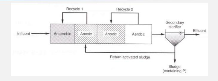
In the modified UCT process shown on the second diagram, the return activated sludge is directed to an anoxic reactor that does not receive internal nitrate recycle flow. The nitrate is reduced in this tank, and the mixed liquor from the reactor is recycled to the anaerobic tank. The second anoxic tank follows the first anoxic tank and receives internal nitrate recycle flow from the aeration tank to provide the major portion of nitrate removal for the process (e) VIP
