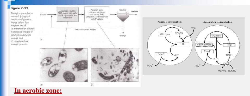
The PHB stored in aerobic zone is used as source of organic carbon for new cell growth and thus providing energy.
