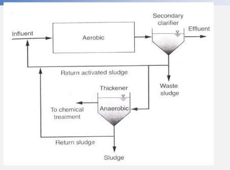
In PhoStrip process, phosphorus - removal efficiency depends less on the influent rbCOD concentrations than for other biological phosphorus – removal processes Can be easily incorporated into exsiting activated sludge plants.
