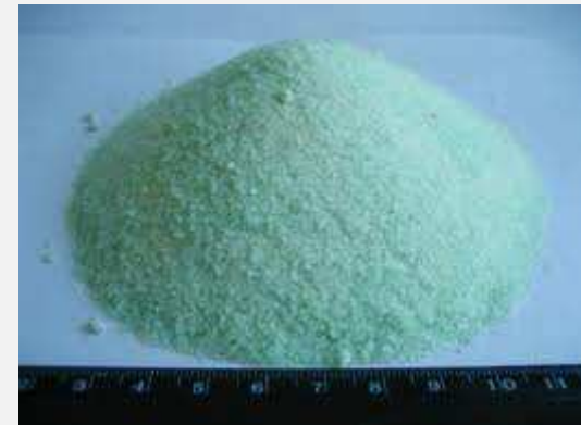
Ferrous sulfate (copperas)
