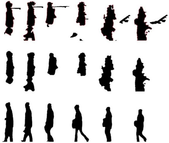
Fig. 6. Processing in the  $x-y$  domain: Top row shows the original segmentation maps for frames 5, 9, 20, 85, 102, and 110 from left to right. Middle row shows the segmentation maps after  $x-y$  domain processing. Bottom row shows the ground-truth segmentation maps for the same frames.
