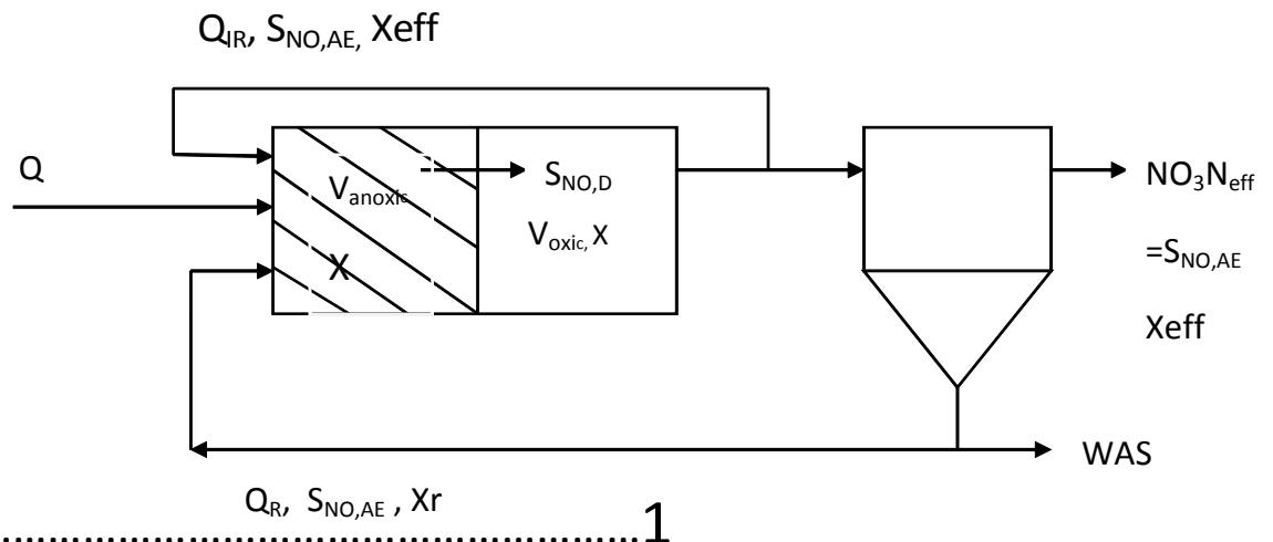
Making a microorganism mass balance for a completely mixed flow reactor with recycle:
