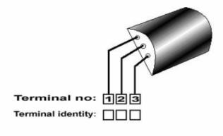
1. Set the selector of the multimeter to the  $10k\Omega$  range. Connect multimeter probes as indicated in the table, and fill the readings.
