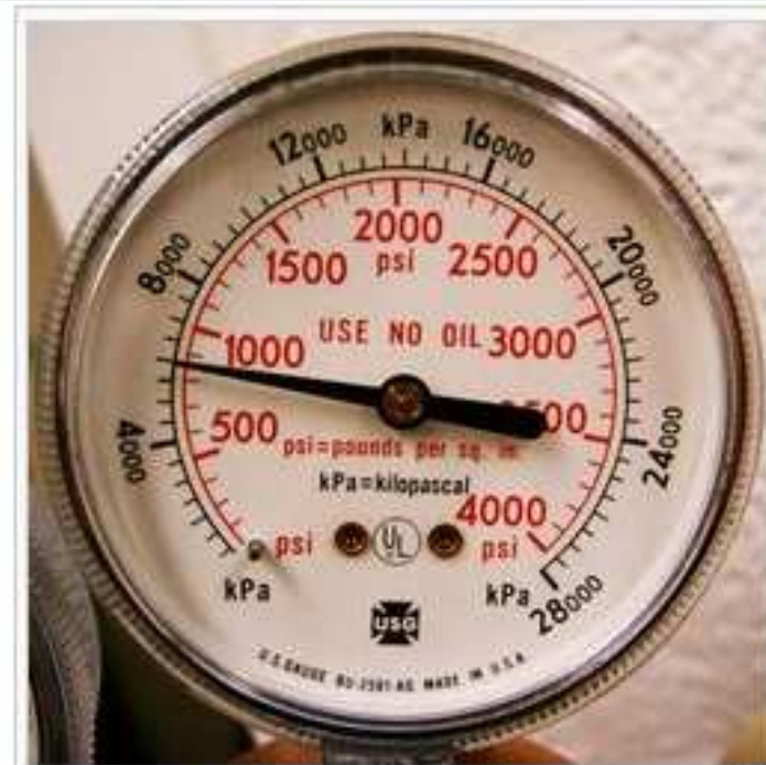
A pressure gauge reading in psi (red scale) and kPa (black scale)
