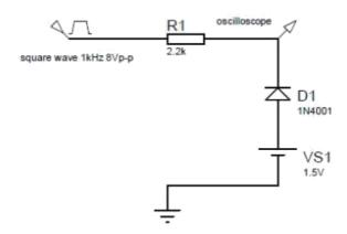
7. Using the measured values of  $V_T$ , E, and R, calculate the output voltage  $V_{\text{OUT}}$ . Show all steps of your calculations. Note that the output voltage will have different values for each input values of +4 V and -4 V)
