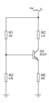
Using the beta determined before, calculate the theoretical levels of  $V_B, V_E, I_E, I_C, V_C, V_{CE}$  and  $I_B$  for the new circuit. Fill results table on next page.
