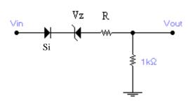
3) Consider the voltage regulator (or voltage reference) circuit. The zener diode has maximum power  $P_{ZM}$ =0.25 W. To keep Vout=4.7 V. for the input voltage rage 9<Vin<20, what must be the range of the resistor R?
