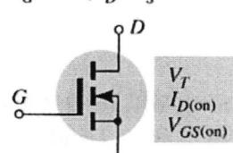
$$I_D = k (V_{GS} - V_{GS(\text{Th})})^2$$
