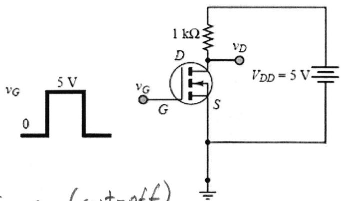
For  $v_G = v_{GS} = 0 \Rightarrow I_D = 0$  (cut-off)
