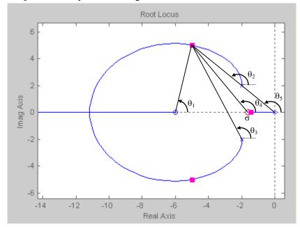
Therefore the required PD compensator is:  $\underline{G}_{C}(s) = K(s+1.56)$ .
