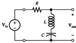
$$G(s) = \frac{V_{out}(s)}{V_{in}(s)} = \frac{Ls + \frac{1}{sc}}{R + Ls + \frac{1}{sc}} = \frac{LCs^2 + 1}{Lcs^2 + Rcs + 1} = 1 - \frac{\frac{R}{L}s}{s^2 + \frac{R}{L}s + \frac{1}{Lc}}$$
