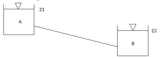
$$z_{A} + \frac{v_{A}^{2}}{2g} + \frac{P_{A}}{\gamma} = z_{B} + \frac{v_{B}^{2}}{2g} + \frac{P_{B}}{\gamma} + h_{L}$$
