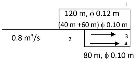
$$(T = 20^\circ\text{C}, e = 0.026 \text{ mm}, v = 1.003 \times 10^{-6}) \rho = 998 \text{ kg/m}^3$$
