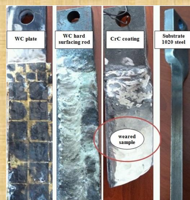
Fig. 2. The coated and uncoated states of mixer knives used in service conditions.
