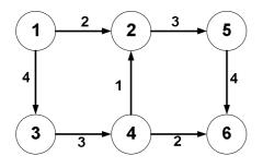
Node 1 is source and Node 6 is sink. Numbers on links are capacities.
