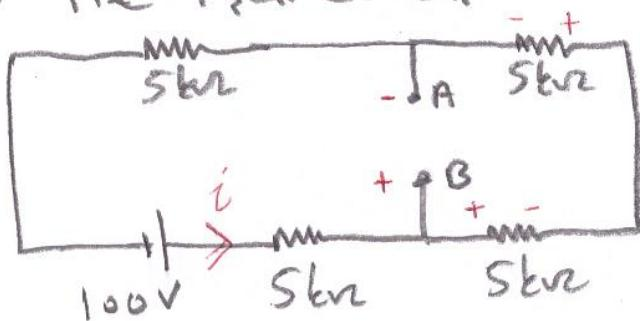
$$i = \frac{100\text{V}}{10\text{k}\Omega} = 5\text{ mA}$$
