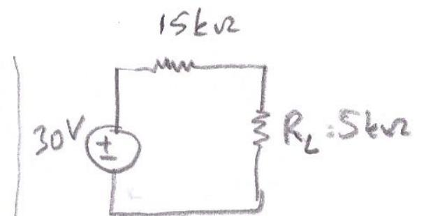
$$i = \frac{30\text{V}}{20\text{k}\Omega} = 1,5\text{ mA.}$$
