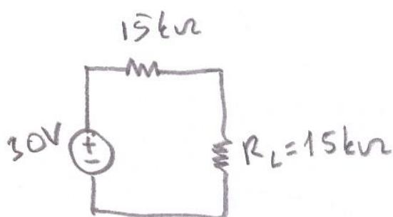
$$i = \frac{30\text{V}}{15\text{k}\Omega} = 1\text{ mA.}$$
