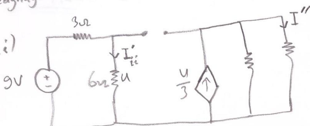
$$I_{ii} = \frac{9}{9} = 1 \text{ A}, \quad U = 6 \text{ V}$$
