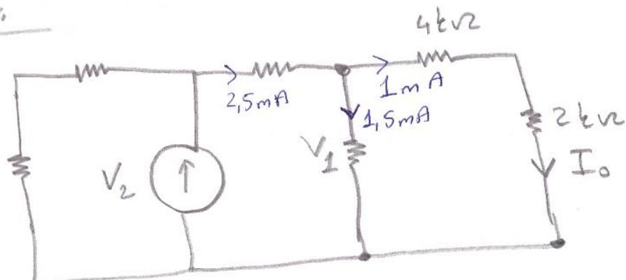
$$V_1 = 1\text{mA} \cdot (4000 + 2000) = 6\text{V}$$
