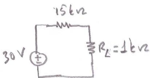
$$i = \frac{30\text{V}}{16\text{k}\Omega} = 1,875\text{ mA}$$
