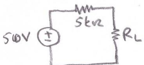
a)  $R_L = 5\text{k}\Omega \Rightarrow i = \frac{50\text{ V}}{(5+5)\text{k}\Omega} = 5\text{mA}$
