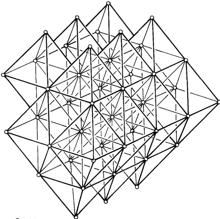
Figure 10.4 Octet truss.
