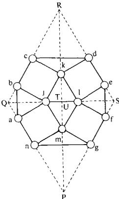
**Figure 6.A.4** A nonrigid framework obtained as the end result of a series of projections of the framework in Figure 6.A.3.
