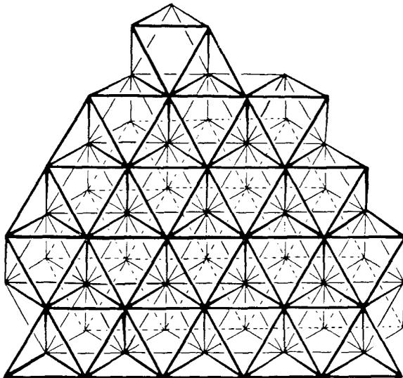
Figure 10.24 Isotropic vector matrix and octet truss.
