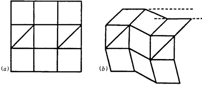
Figure 4.59 By the lemma the elements of row 2 are perpendicular to the elements of columns 1 and 3.
