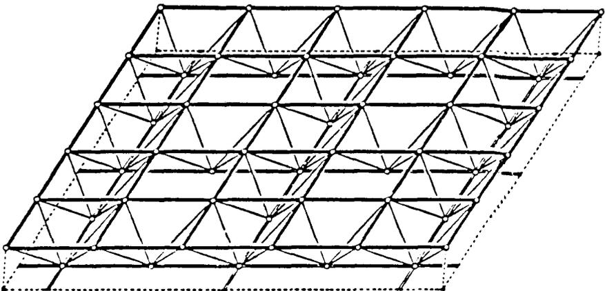
Figure 10.5 Planar arrangement of an octet truss into half octahedrons and tetrahedra.
