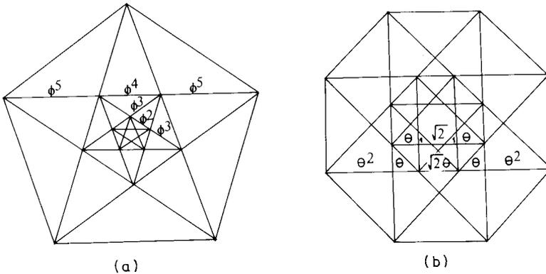
**Figure 3.18** (a) Star pentagons at decreasing scales. The ratio of lengths from scale to scale is  $\phi^2:1$ . The edges of the star cut each other in the golden section. (b) Star octagons at decreasing scales. The ratio of lengths from scale to scale is  $\theta:1$ . The edges of the star cut each other in the ratio  $\sqrt{2}:1$ .
