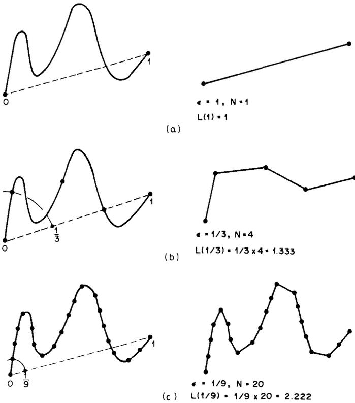
**Figure 2.23** Determination of the length  $L$  of a curve spanning  $[0, 1]$  by approximating the curve with  $N$  line segments. (a) Representation of curve at scale of  $\epsilon = 1$ ; (b) representation of curve at scale of  $\epsilon = 1/3$ ; (c) representation of curve at scale of  $\epsilon = 1/9$ .
