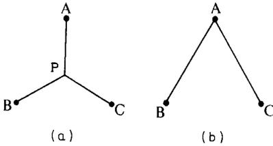
Figure 6.2 Minimal networks for three points. (a) Minimal network; (b) a nonminimal network.
