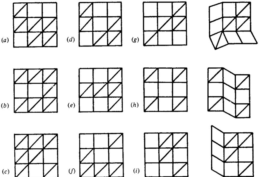
Figure 4.56 Some bracings of a 3 by 3 grid.
