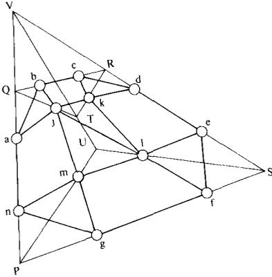
**Figure 6.A.3** A framework formed by truncating a tetrahedron.
