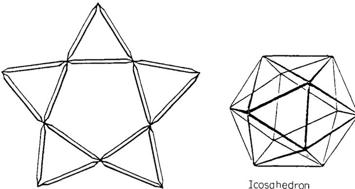
**Figure 7.1** Pattern for constructing an icosahedron dome with marshmallows and toothpicks.
