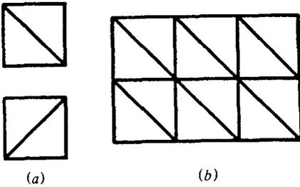
Figure 4.54 Bracing a structure to make it rigid by adding a crossbeam.
