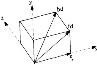
Figure 7.27 The principal directions of a cube.
