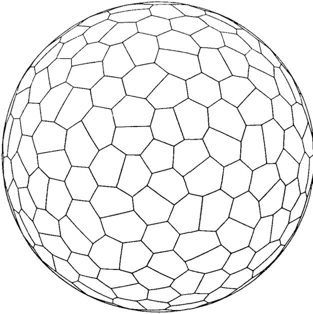
Figure 5.22 Geometric design for a 68-foot radome.
