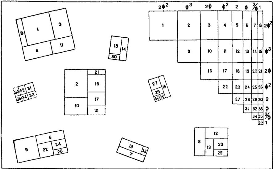
Figure 1.11 A Moduler exercise by Le Corbusier. Eight rectangles are subdivided by Moduler rectangles and coded according to the table in the upper right-hand corner.
