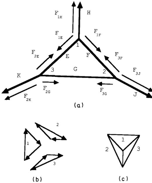
**Figure 6.17** The arrows in (a) show the tensions of a spider web stress on a cell decomposition. The polygons of forces for the equilibria at the vertices (b) are pieced together and rotated 90 degrees to form a convex reciprocal figure (c).
