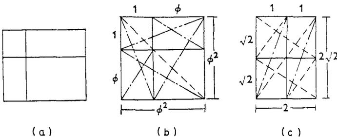
Figure 1.8 A rectangle subdivided by one vertical and one horizontal line into nine subrectangles. The rectangles have (a) all different proportions; (b) three different proportions based on  $\phi$ ; (c) two different proportions based on  $\sqrt{2}$ .
