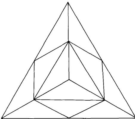
Figure 9.23 Construction of an intersection of three vaults (IV). The edges of the IV must abut with the edges of the three vaults.
