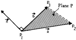
Figure 7.16 The normal vector to a plane.
