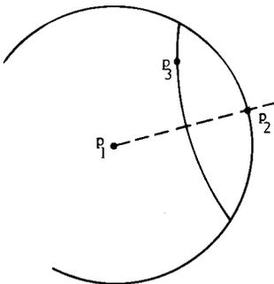
**Figure 7.13** Three noncollinear points on a rigid body.
