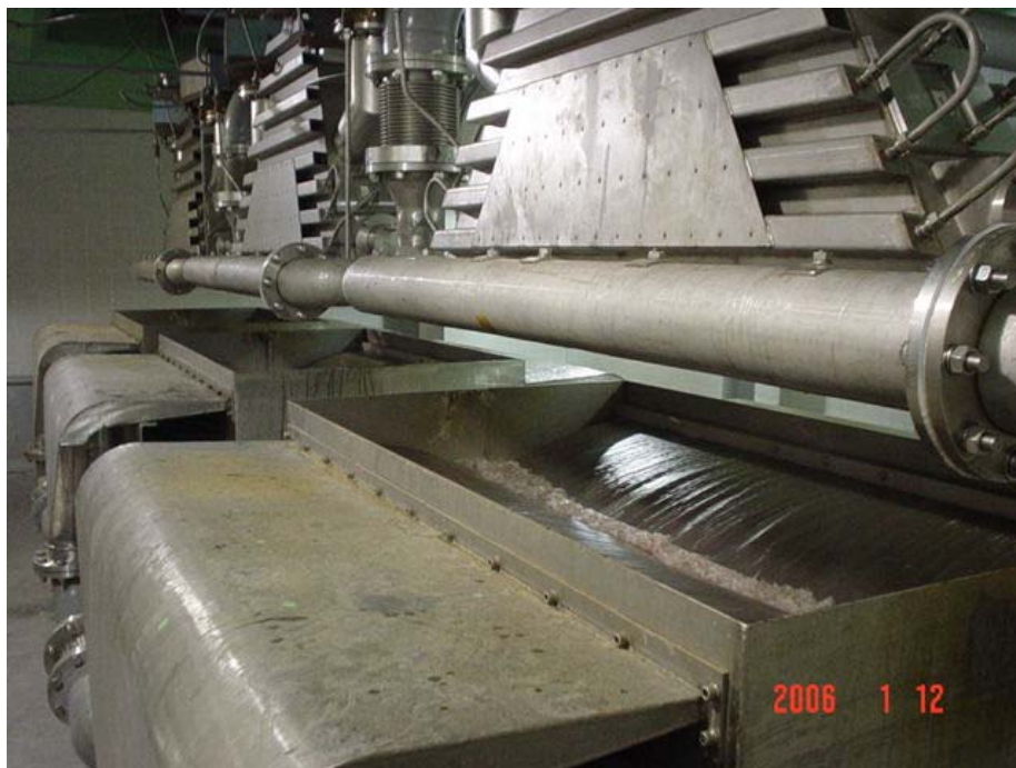
Figure 15. Irradiation of industrial dyeing complex wastewater in the area of Taegu Industrial Complex, Taegu, Republic of Korea (Courtesy of Bumssoo Han [77]).
